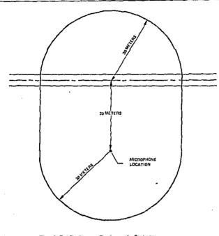
Figure 1, Test Site Clearance Requirement for Stationary Locomotive, Locomotive Past-by, Rail Car Pers-by, and Locomotive Load Cell Test Stand Tetla.
